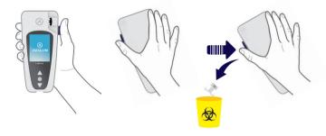
To minimize the risk of contamination, this unique ejection system was designed such as user never gets in contact with a used SmartChip.
