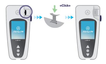
Following Tsmart® insertion, the reader performs required internal quality controls and prepares to perform the test, which may include preheating for instance. Quality control of the Tsmart® is automatically performed. In case an error occurs during this initialization phase, the corresponding error message is displayed on the screen and the Tsmart® must be ejected (See Section 9 «Error messages»): you will have to repeat the process, using another Tsmart® when required.
