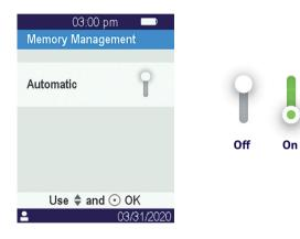
When automatic memory management is deselected, a new option called «Results deletion» is made available as part of submenu «Measurements». This option allows to delete older results starting from the oldest one by using the navigation buttons.
