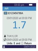
Press again the middle button to display the result which, depending on the test, may be displayed in several screens. When several units are available, use triangular navigation buttons to select the desired one.
