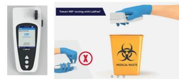
When the test is complete, the LabPad® beeps at regular intervals until the Ksmart® is ejected. To dispose of the Ksmart®, press the black button on the side of the instrument.
